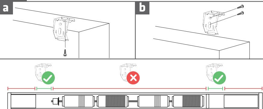
**2** **DK/NO/SE:** Hold gardinets profil mod beslagets forreste kant og tryk opad bagtil. **EN:** Hold the curtain profile against the front edge of the bracket and push up towards the back.
